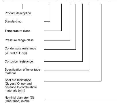
Properties of a multi-wall metal chimney system
